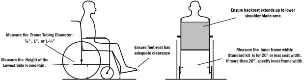
To determine the correct interface bracket measure the **tubing diameter**. Also measure the **height of the lowest frame tubing**, running front to back, from the floor. If the seat width is in excess of 20", measure the span between the inside of the side frame rails.
