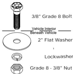
Ensure that **all fasteners** for both the BL-6290 base lock and the wheelchair interface bracket are **in place** and have been **tightened firmly**.
